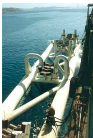
Firing line on stinger
